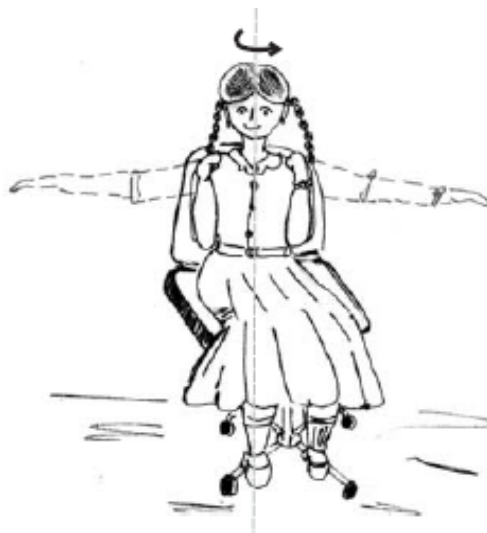
Fig 7.36 (a) A demonstration of conservation of angular momentum. A girl sits on a swivel chair and stretches her arms/brings her arms closer to the body.
